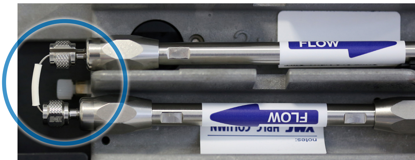
Figure 1: Coupling of two YMC-Triart C18 ExRS UHPLC columns using the dead volume free MarvelX™ connector.
